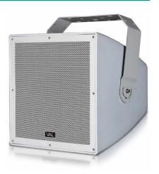
ing bracket is sprayed with low-carbon steel, which can meet all- weather use. It features a  $1\times15$ " ferrite mid-bass driver and coaxially mounted  $1\times3$ " voice coil HF driver on a  $60^{\circ}\times25^{\circ}$  waveguide. The WP15CXL unique design allows it to be used as a standalone speaker or in arrays of upto 4 speakers with additional flying hardware.
