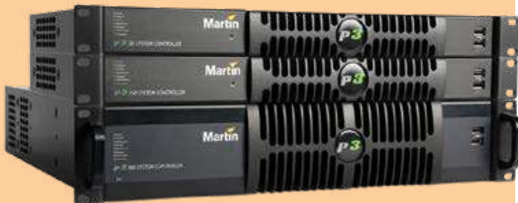
Martin P3 System Controller Software Version 5.3.0 supports NDI protocol with network driver
