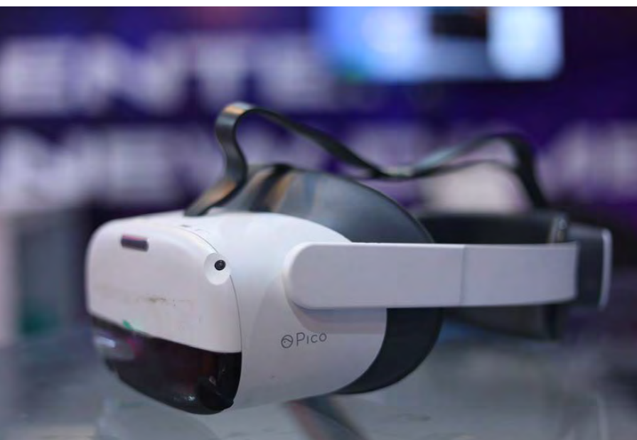
The PICO VR Headset, designed to deliver an immersive experience with 6DoF positioning, Qualcomm XR2 platform, 4K HD screen, and more
