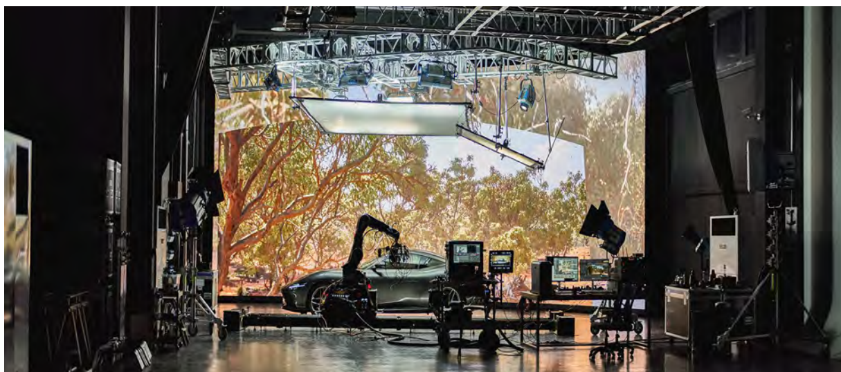
XR space, equipped with ROE Visual Black Pearl panels, Brompton Technology LED processing, Mark Roberts Motion Control cinebots, Unreal Engine, and disguise media server hardware.
