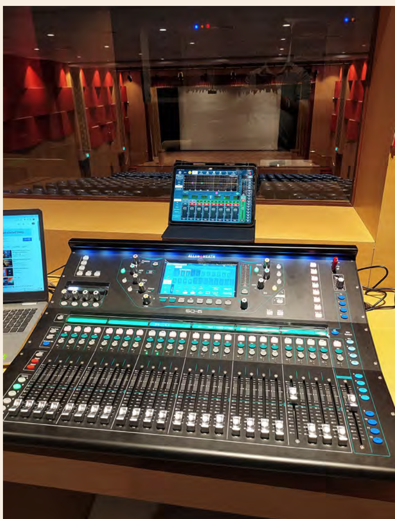
Allen & Heath's SQ6 - 48 channel / 36 bus digital mixer coupled with One DX168 96kHz portable expander installed in the Sound Room
