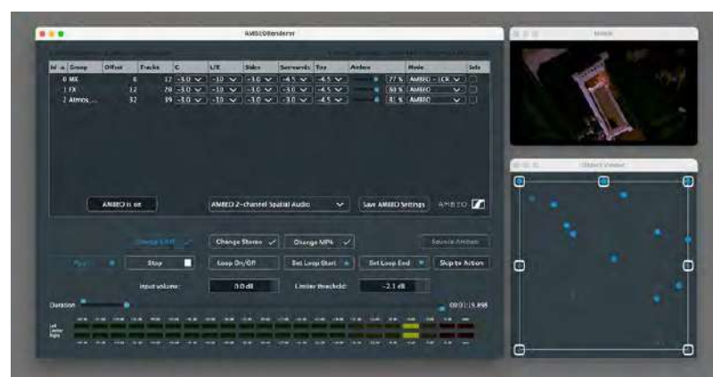
The preview tool of the AMBEO 2-Channel Spatial Audio rendering software. The Object Viewer window at the bottom right shows fixed loudspeaker positions at the edges and individual renderings as blue dots. Pale dots are elevated sound sources
