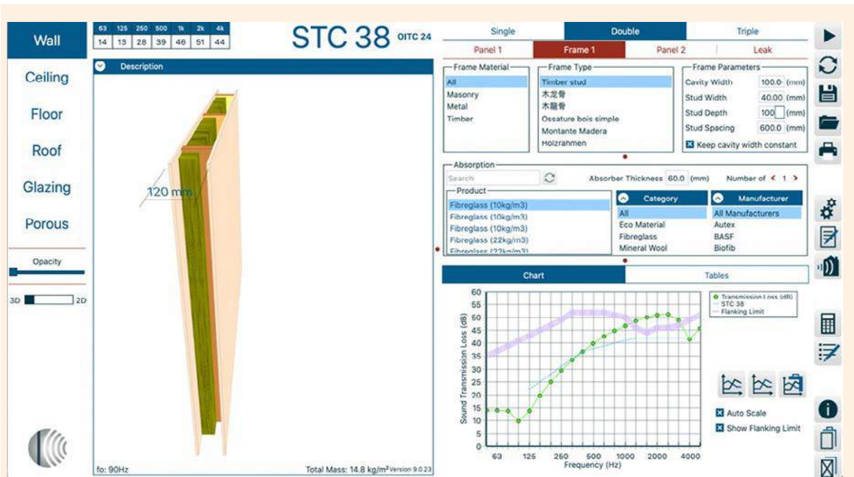
Fig. 2: Partition design with INSUL
