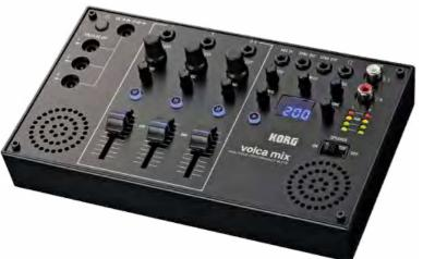
compresses the high-frequency range according to level changes of the low-frequency region, as well as a side chain effect that's indispensable for dance music. Use these to dynamically vary the mix, adding a professional feel to live performances with the volca. The volca mix comes with AC adapter, DC-DC cables, and audio cables included.
